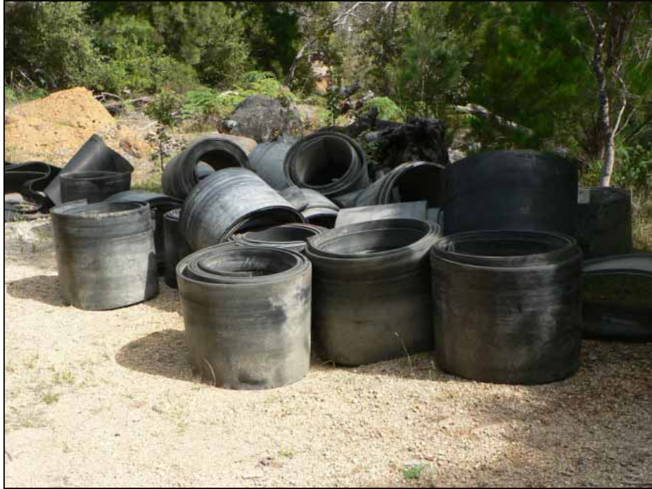
IMAGE 10. TRACK MATTING IN ROLLS PRIOR TO INSTALLATION WEST CAPE HOWE NATIONAL PARK
